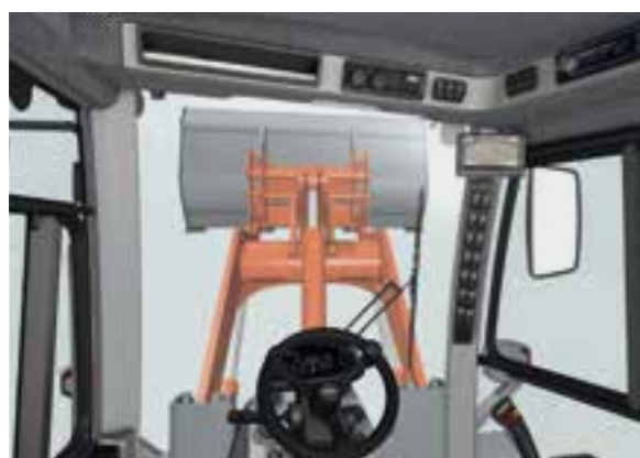
Front: Unimpeded view from the top to the floor, unobstructed by the steering column.
