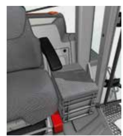
Designated space for euro boxes so the driver can keep documents or private items in the vehicle – ideal for multi-shift operation.
